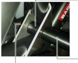
USE THE 25 mm THICKNESS INSIDE THE BRACKETS AND MOUNT THE 55 mm THICKNESS ON THE EXTERNAL SIDE.
