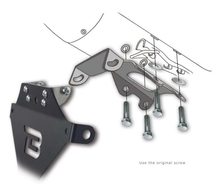
REMOVE THE ORIGINAL LICENCE PLATE AND APPLY, INTO THE SAME HOLES, THE BARRACUDA LICENCE PLATE USING THE SAME SCREWS REMOVED FROM THE ORIGINAL LICENCE PLATE (LOOK THE PICTURES)
