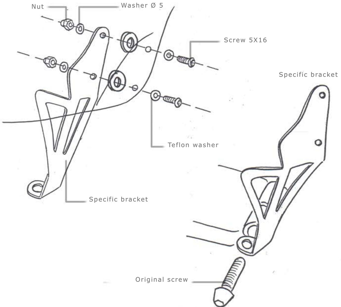
APPLY THE TWO BRACKET ON THE STEERING PLATE USING THE ORIGINAL SCREW. FIX THE WINDSHIELD/SCREEN ON THE TWO BRACKET WITH THE 5X16 SCREW LIKE DESCRIBED INTO THE PICTURES. FOUND THE CORRECT POSITION OF WINDSHIELD/SCREEN, LOCK ALL AND USE THE 4 RUBBER WASHER BETWEEN THE IRON BRACKET AND WINDSHIELD/SCREEN
