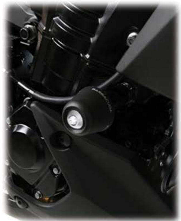
SEARCH AND FIND THE FIXING POINT ON THE MOTORBIKE BEFORE START TO MOUNTAIN, USE THE SPECIFIC THICKNESS AND BOLTS LIKE DESCRIBED IN THE PICTURE (SO YOU CAN GET THE RIGHT PROMINENCE FROM THE MOTORBIKE).
